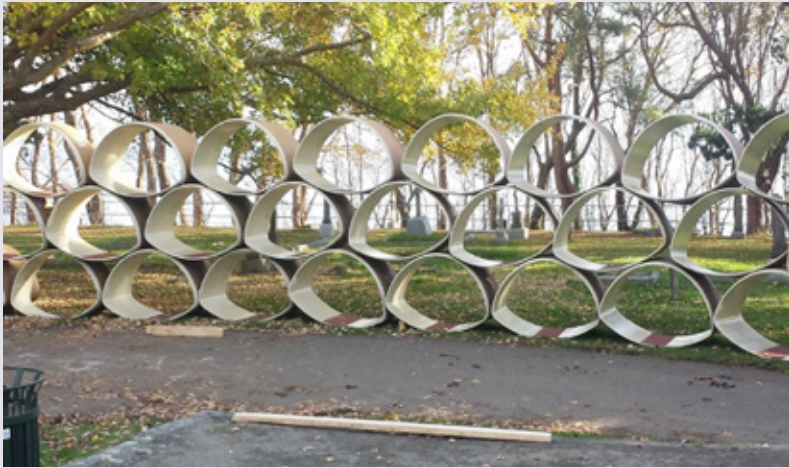
Glass Reinforced Plastic (GRP) segments are becoming more widely used for sliplining
